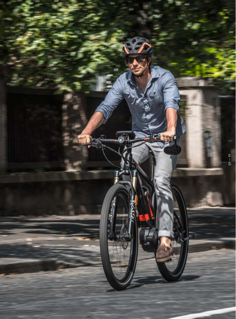
Nyon is the first E-Bike computer that unites all functions on one device. Whether it's information about speed, cadence or range, personal fitness analysis or GPS navigation, it's all catered for by the Nyon. The intuitive handling is made possible by a 5-way joystick on the device itself, or via a separate control on the handlebar.
