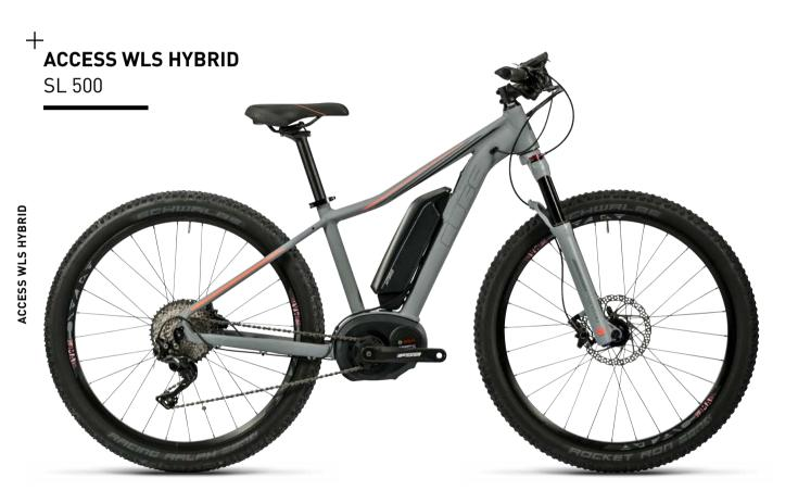
The Access WLS Hybrid is more than just a mountain bike with a battery. We developed our Agile Ride Geometry with shorter and sloping top tube. At the development we took in to consideration every detail and constructed a frame with low weight but that is stiff and robust. The frame transfers the power of the new Bosch CX Drive on the trail, with up to 75Nm this e-mountain bike drive is well in the upper class.
